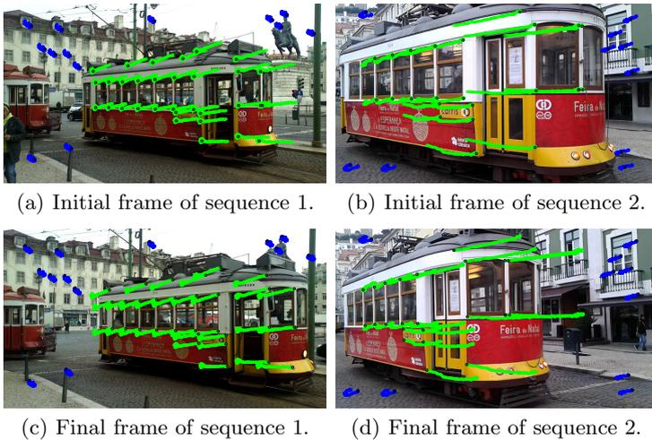
**Fig. 4.** Initial and final frames of the two sequences in the experiment with independently moving cameras. The evolution along time of features in the tram and features in the background are represented in green and blue, respectively. The black dots identify the position of the features at the time of acquisition of the presented frames.
