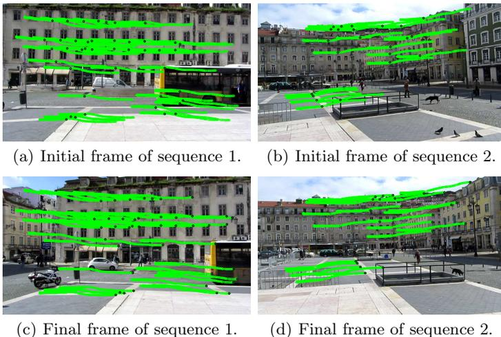
**Fig. 2.** Initial and final frames of the two videos in the experiment with jointly moving cameras. Green dots represent the evolution over time of features on the background, and black dots identify their position at the time of acquisition of the presented frames.
