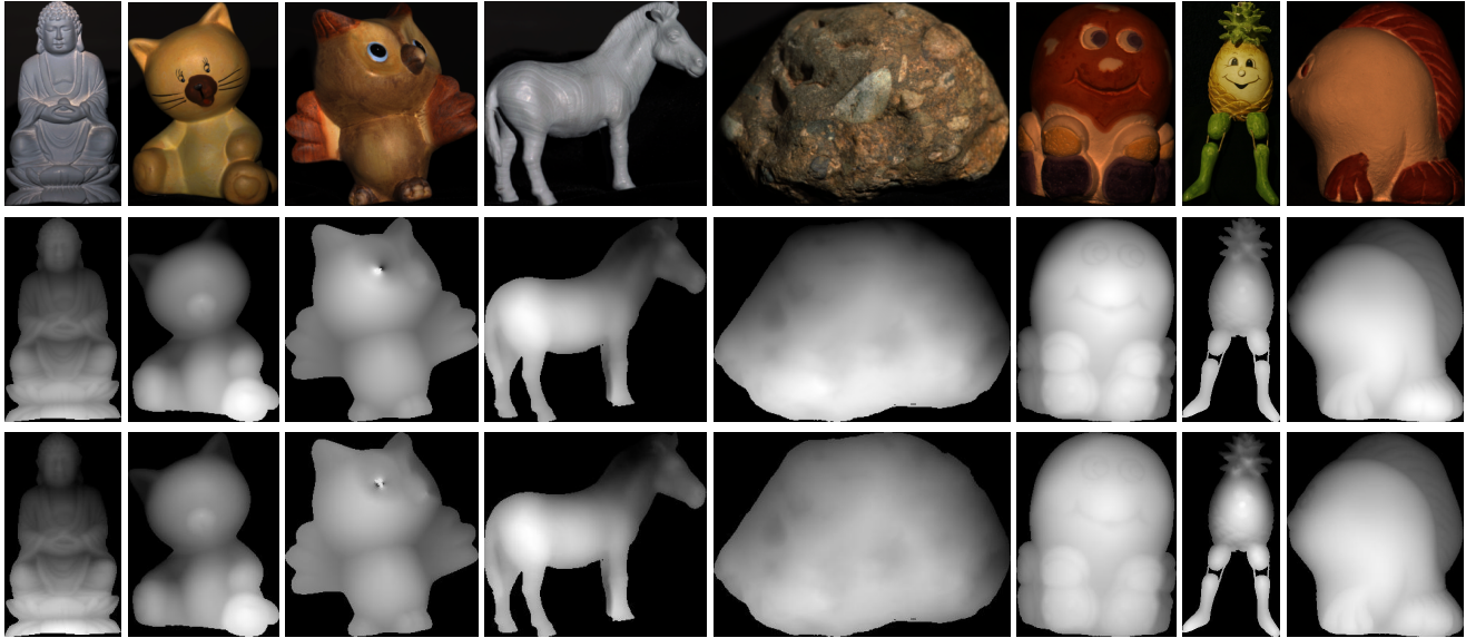
Figure 6. Reconstructed depth maps. Top row: One of the input images. Middle row: Graylevel-coded depth map reconstructed with calibrated photometric stereo. Bottom row: Graylevel-coded depth map obtained with our method.
