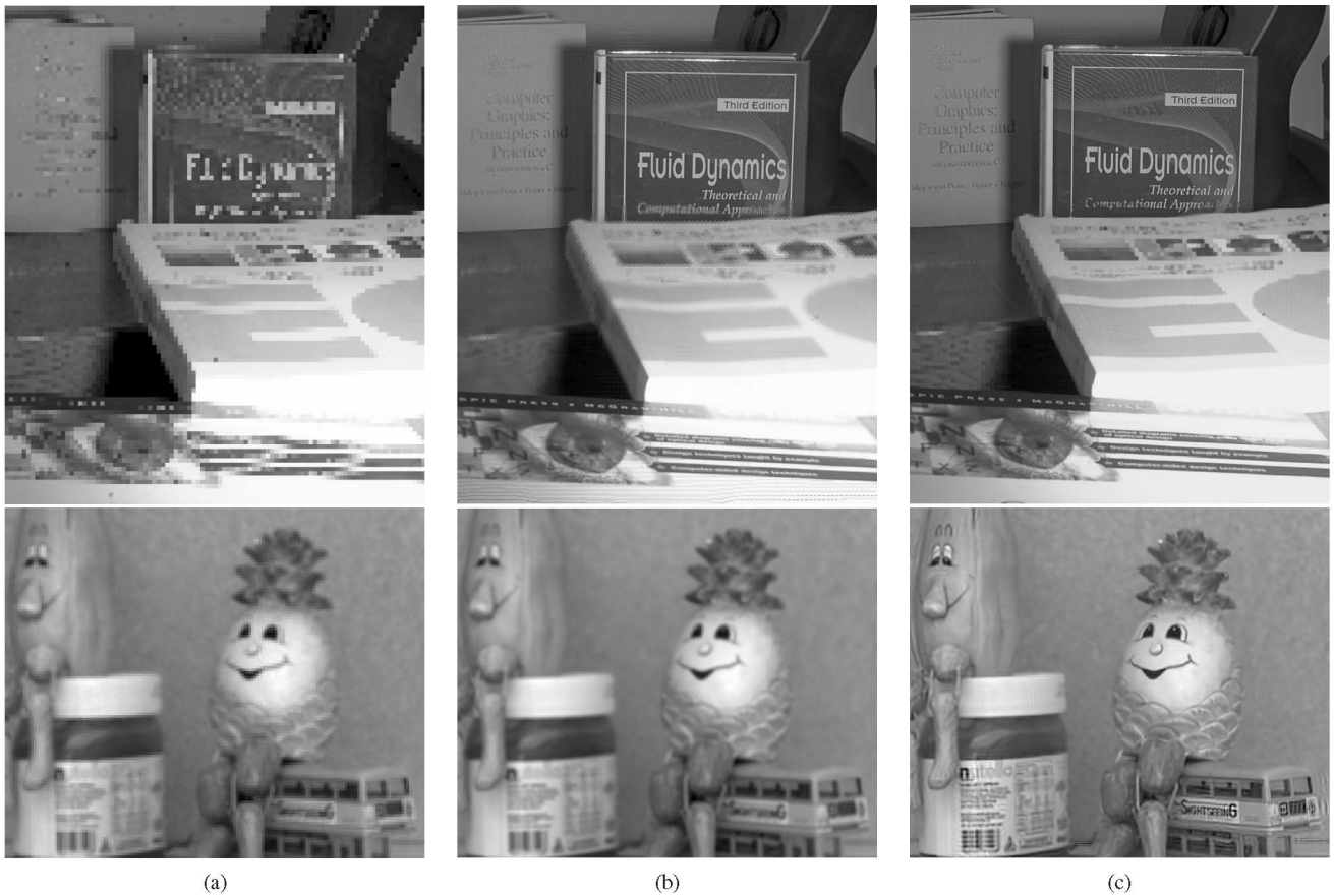
Fig. 18. Superresolution on real data Top row: Data from Georgiev and Lumsdaine [22] ( \kappa = 1.4 ); Bottom row: “puppets” data set ( \kappa = 3 ). (a) Nearest-neighbour interpolation of one view. (b) High-resolution view using method of Lumsdaine and Georgiev [6]. (c) View superresolved with our method.
