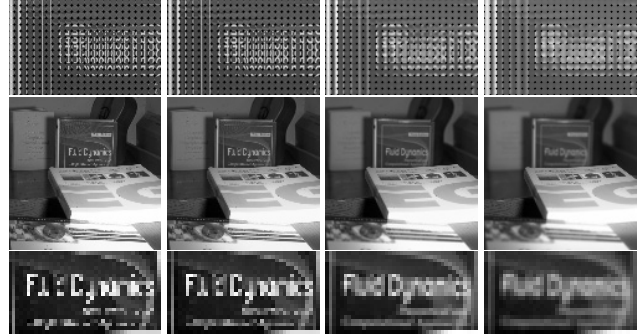
Figure 9. Filtered subimages (filter size increases from left to right). Top row: Close up of a few microlens subimages. Middle row: Corresponding filtered full view. Bottom row: Magnified detail of the view.
