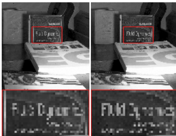
Figure 1. Example of aliasing in plenoptic views. Left: One view extracted from a plenoptic image (courtesy of [6]) with one enlarged region shown at the bottom. Right: Another view extracted from the same data set (along the horizontal axis). Notice the apparent aliasing affecting these views. Establishing correspondence for depth inference in these views is therefore prone to errors.
