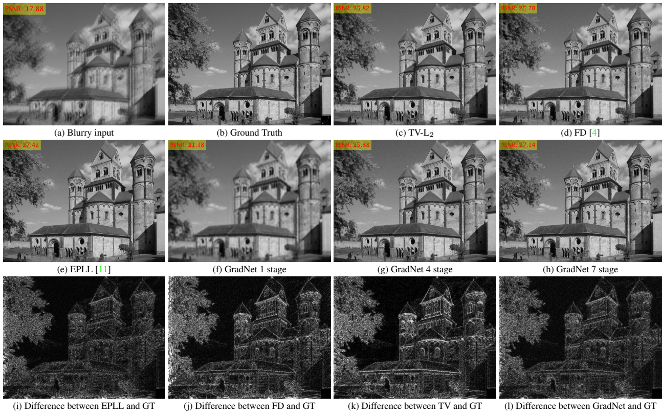
Figure 7. Results for the 1% noise case (best viewed on screen). PSNR results are also shown at the top left corner of the estimated images.
